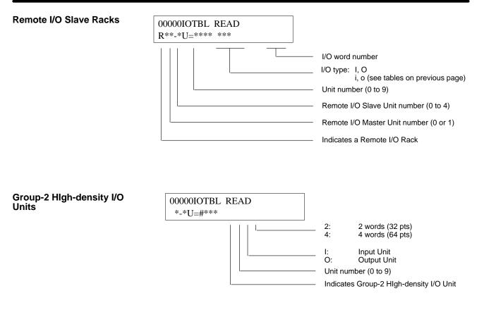
**Note** Group-2 HIgh-density I/O Units will not be displayed in the I/O table when it is displayed using LSS (host computer). Four asterisks (\*\*\*\*), indicating no Unit, will be displayed instead.
